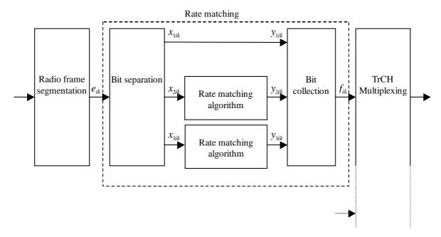
Figure 5: Puncturing of turbo encoded TrCHs in uplink
